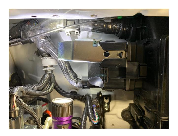
5) install the tray to the 2 factory holes on the side and 3 on the wheel arch holes
