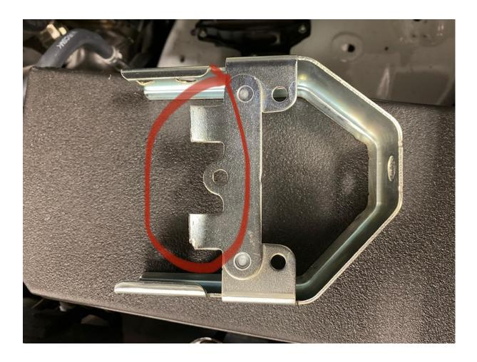
3) You will need to drill a new hole into the bracket to fit the factory 12mm bold thought it. I drilled the left hand side of the bracket shown above and drill the hole closer too the bent it will allow you to use a 12mm with a swivel to secure the bracket back down with the relay box secure back to the bracket
