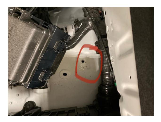
4) Re install the relay box too the bracket and turn the relay box side ways. screw the factory 12mm bolt back into the bottom hole that secured the bracket. It will sit close to the fuse box but won't rub against it
