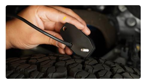
STEP 5 Using the provided M6x25mm allen head hardware, secure the utility light in place using a #4 allen tool and a 10mm wrench.
