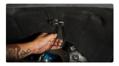
STEP 7 | Connect the light to your power supply. For this install we used the DV8 4 way harness and 60 amp switch wiring harness bundle, part numbers UNWH-01 & UNWH-02.
