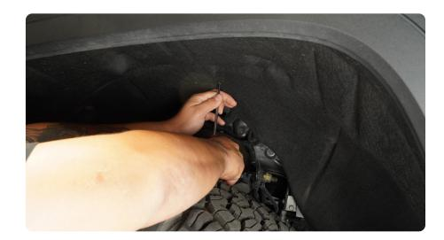
STEP 4 | Place the provided backing on to the back of the light.
