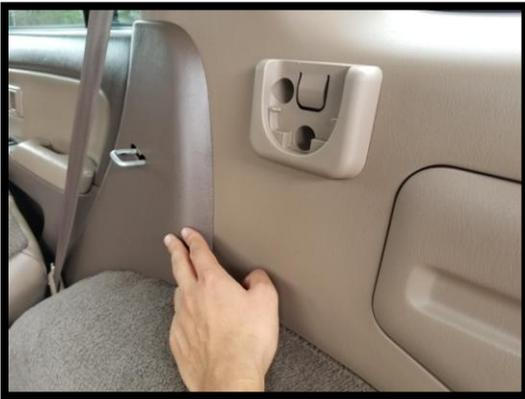
To remove the shoulder panel, the door floor trim must be removed, locate two screws and remove the door floor trim by firmly pulling away.
