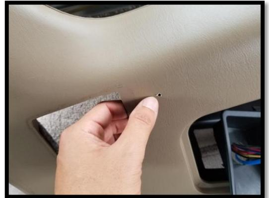
Grab the step bit and drill out to 3/4" hole, stopping periodically to check the fitment of the aluminum spacer. You want a nice snug fit. Don't over drill. Be patient.
