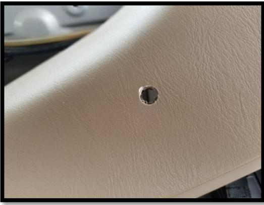
Test the spacer for a nice, snug fit.
