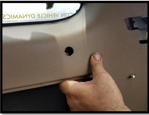
Drill your second hole and install the panel, yes. **INSTALL** it. Make sure all the fasteners clip in place. Make sure it doesn't wobble. Make sure it is set to **STAY**. You will see why. This is important.
