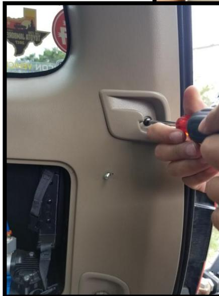
remove cargo cover brackets, removing the
