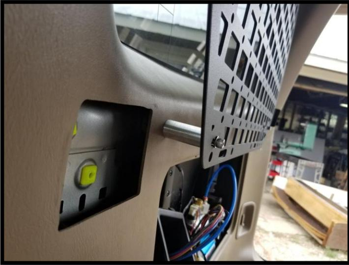
Next make sure your friend is holding the panel to where the brackets are away from the window - I have it about a 1/4" clearance.
