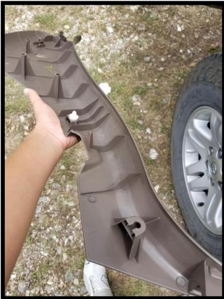
The main cargo panel can now be removed. In this case, the passenger side:
