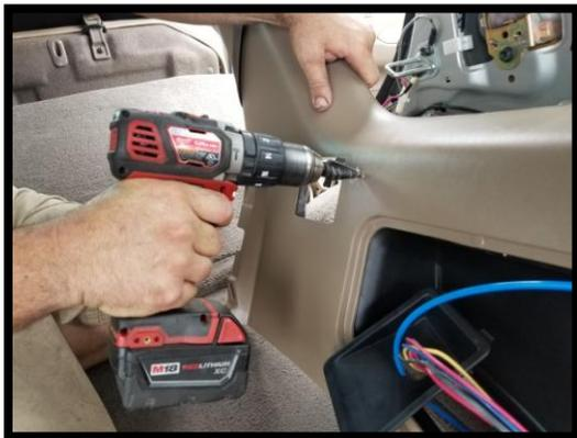
You can barely see the rim of the fastener seat thru the hole. Use it to make sure you are centered.
