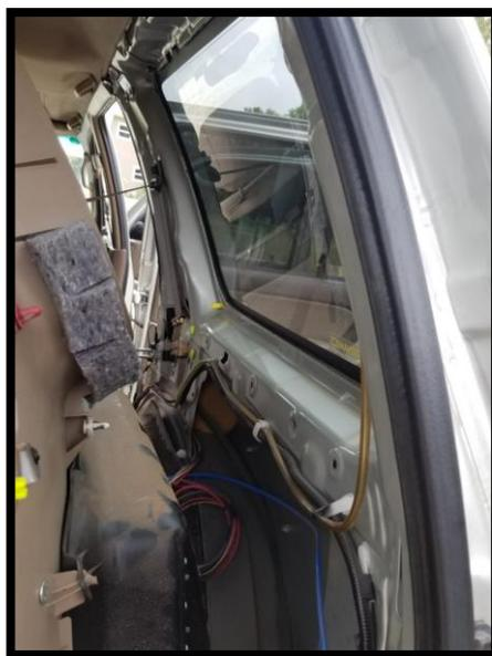
We will now locate the TWO outer holes where the trim fasteners push into. In the picture below, you will see four holes below the window. It is the two outer holes.
