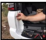
5. Remove the 3 bolts holding the plastic valance in the tire carrier area. This will allow you to gain access behind the bumper.
