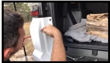
4. Start drilling using the pilot bit. Then use the step bit to drill the whole large. Go slow and stop to check the fit of the screw.
