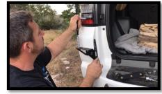
3. Mark desired location with a Sharpie. Only mark the top hole and then center punch the hole.
