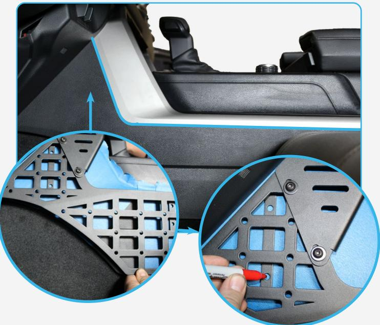
*Pro Tip: Install the bridge to the side molle panels and use a level to ensure that fitment is precise*
