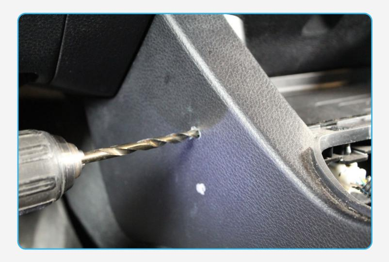
*Pro Tip: Using a tape measure, mark the drill bit with a Sharpe or wrap tape around the bit to a 1/4"*
